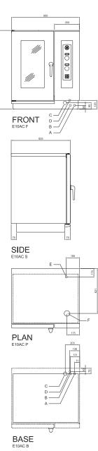
A = WATER CONNECTION R<sup>3</sup>/<sub>4</sub> (SOFTENED WATER) refer to installation
